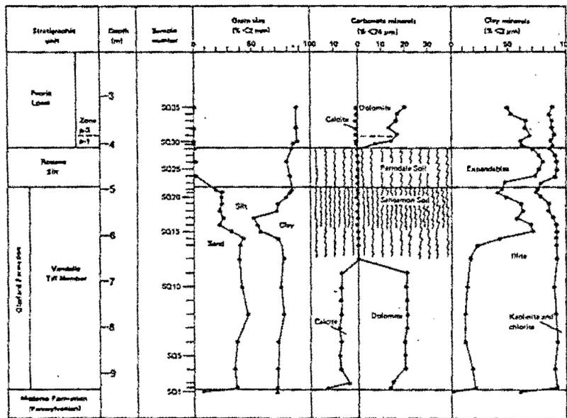
Figure 22. Grain sizes, carbonate-mineral content, and clay mineralogy of the Athens South Quarry Section.
