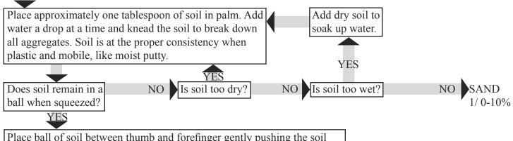
Place ball of soil between thumb and forefinger gently pushing the soil with the thumb, working it upward into a ribbon. Form a ribbon of uniform thickness and width. Allow the ribbon to emerge and extend over the forefinger, breaking form its own weight.
