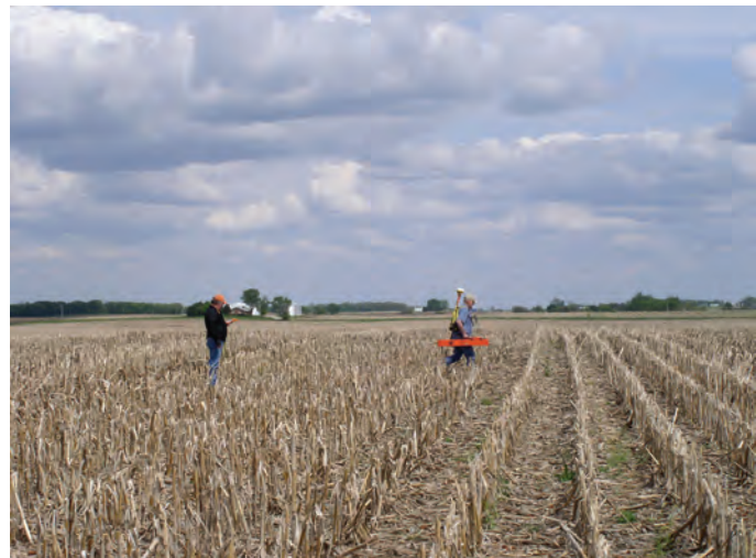
Left to Right: Dan Withers is taking GPS points while Jim Doolittle is taking EM 38 readings while transecting across corn stalks.
