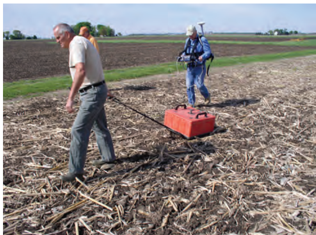
Left to Right: Roger Windhorn, Dan Withers, and Jim Doolittle run a ground penetrating radar test on a terrace area.
