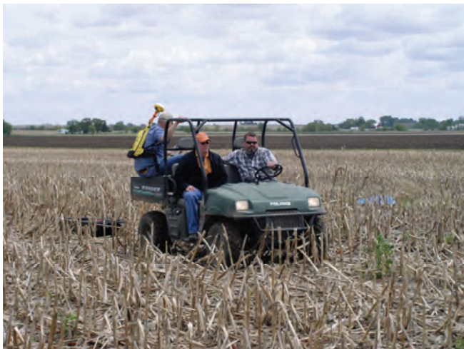
Left to Right: Jim Doolittle, Dan Withers, Tim Malone (DC Tazewell Co.) pull the EM 38 in a sled across corn stalks
